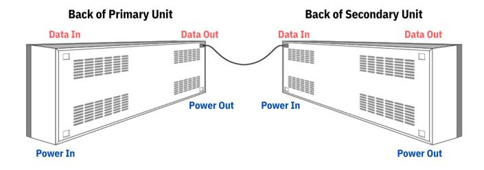
Locate the quick access data connection ports on the Primary unit and Secondary unit. Firmly seat the cable to ensure a solid connection. Gather and zip tie any loose cable. The **Input Data Port** is located on the left side when looking at the back of the unit.
