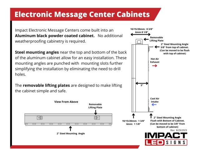
A 2" x .125" thick steel mounting angle runs the length of the top and bottom of each Impact single cabinet enclosure EMC. This design provides tremendous flexibility in mounting.
